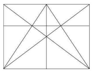
6. Draw a vertical line through the intersecting point and the diagonal line from the vertical to connect the horizontal line from step 5.
