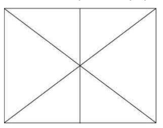
4. Draw a second set of diagonal lines from the lower corners to the top of the centerline.
